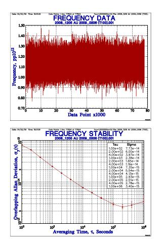
Figure 8. PHM QM1 frequency data and frequency stability (with drift)
