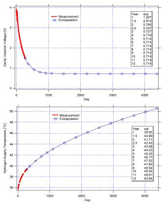
Figure 7. TMs (cavity varactor voltage and hydrogen supply temperature) on QM1 lifetime test with prediction on 12 years
